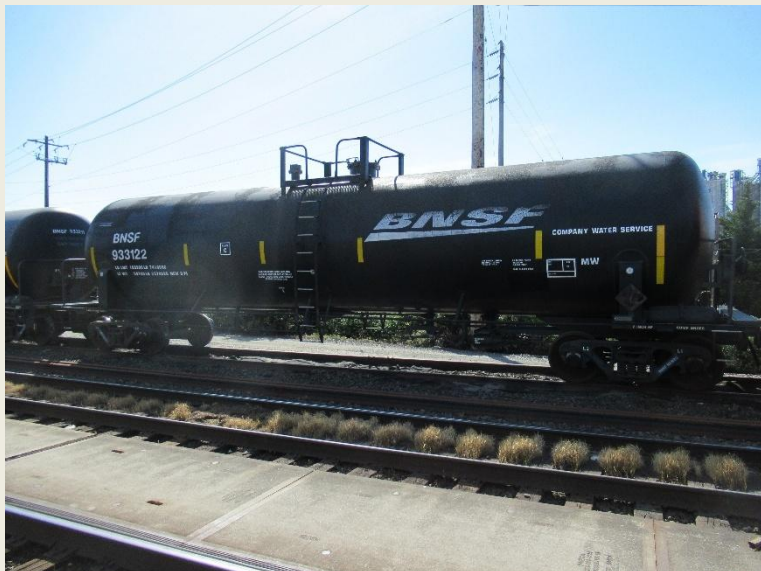
Pictured left is a tank car for water service.
