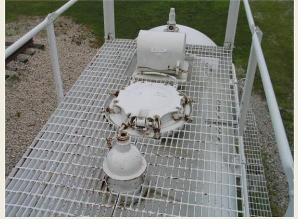
Photo #22 – shows a “Top Operated Bottom Outlet Valve” on a low-pressure tank car. It is also known as a “TOBOV” valve. It works to open a valve or drain on the bottom on a the bottom of a tank car.
