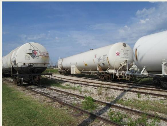
Photos #7, #8, #9 and #10 – show on the left side as you face the tank car the “reporting marks” or “letters and numbers” that are specific for that car. On the right side as you face the tank car you will find the “specifications plate” or important details for the tank car relating to construction, testing and certain parts.
