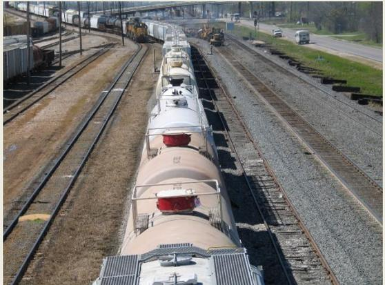
Photo #21 – shows equipment and valving on top of a low-pressure tank car used in the unloading and loading of a tank car.
