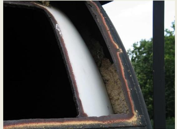
Photos #12 and #13 – show the differences between a “jacketed” and “non jacketed” tank car. You can see in one case how the bolster is welded to the tank. In the other photo that is covered up by the “Jacket”.
