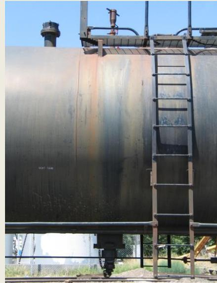
Photo #23 – shows the equipment used for loading and unloading a tank car transporting corrosive liquids. The safety relief equipment is also shown.
