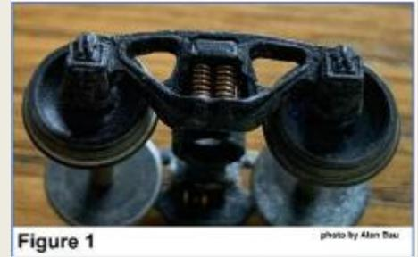
The change from plastic wheels to metal ones is desirable for a number of reasons ie: current pick-up, lower tendency to accumulate crud, better rolling capability, to name a few.
