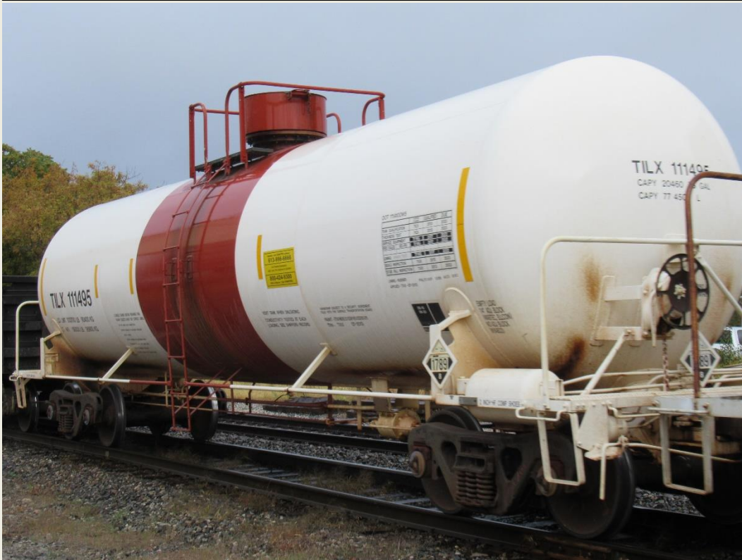
DOT-111 CPC1232 Tank Car (half external head shield and valve protection)
