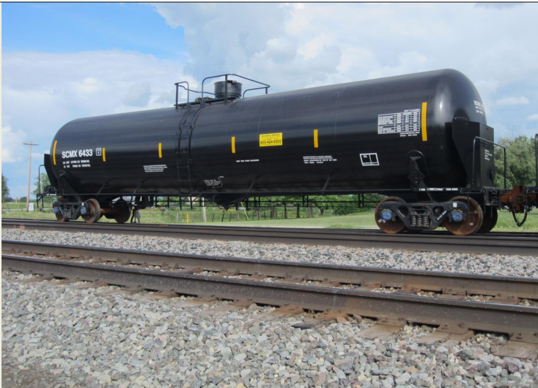
DOT-111 CPC1232 Tank Car (half external head shield and valve protection)
